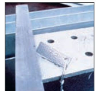
Figure 39: Tag affixed with a minimum #9 gauge steel wire
