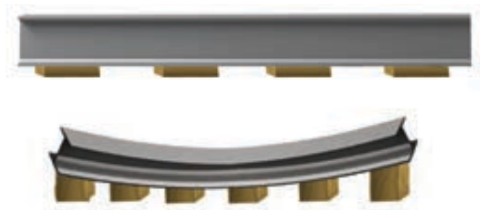
Figure 14: Avoid leaving mid-portion of products unsupported, products should be laid with supports to prevent sagging or to support a camber.
