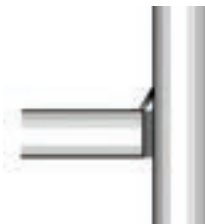
Figure 32: 3/32 inch (2.5mm) gap after welding
