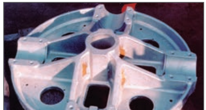
Bare spots due to embedded sand not removed from casting prior to hot-dip galvanizing
